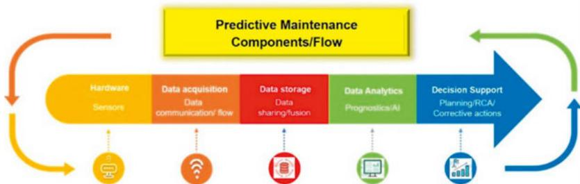
Figure 2: Components and flow chart of predictive maintenance.
