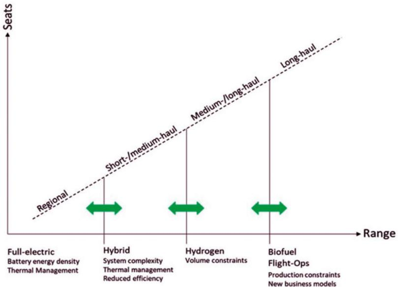
Figure 8: Novel propulsion technologies and their expected operational deployment<sup>15</sup>
