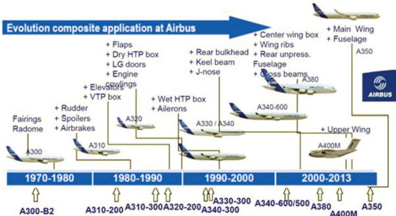
Figure 5: Evolution in composites aircraft applications (Airbus, 2013)
