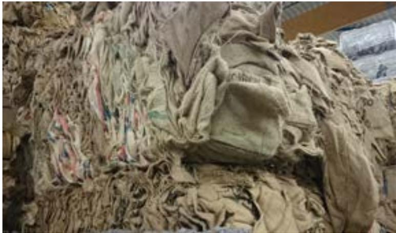
Textile wastestream: jute coffee bags, in which the raw coffeebeans are transported from a worldwide scatter of suppliers to the Starbucks coffee processing factory in the Amsterdam harbour. Approx. 240 tons/yr.
