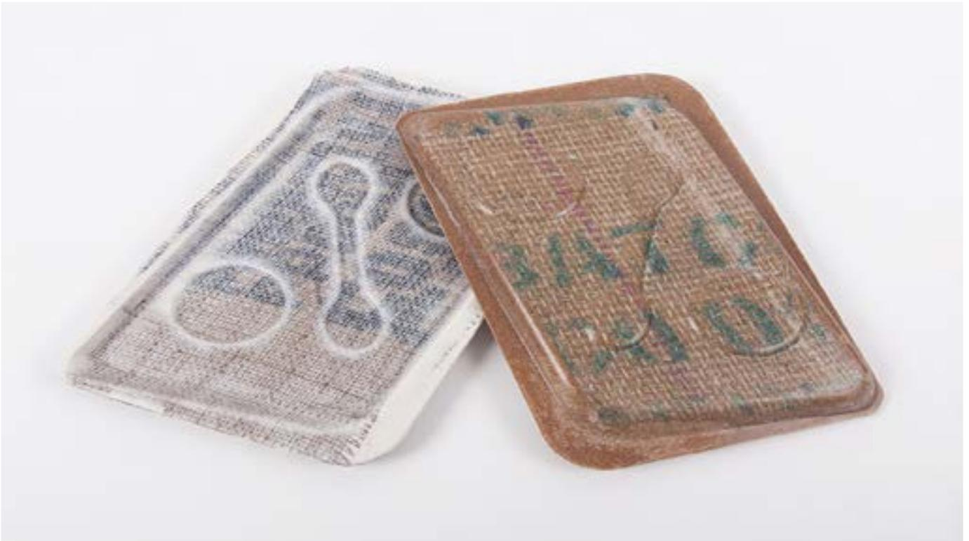
Serving trays made from a.o. jute mats and Solanyl (PLA/TPS) Hot pressing
