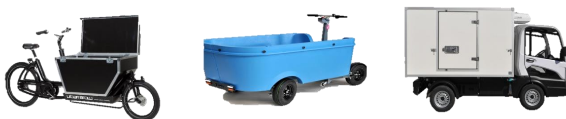
Figure 2 Examples of light electric freight vehicles (v.l.t.r.: Urban Arrow, Stint, Goupil)
