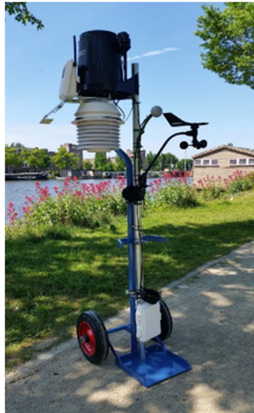
Fig. 2 Mobile weather station. Davis Vantage Pro2 instrument installed on a wheel hand cart
