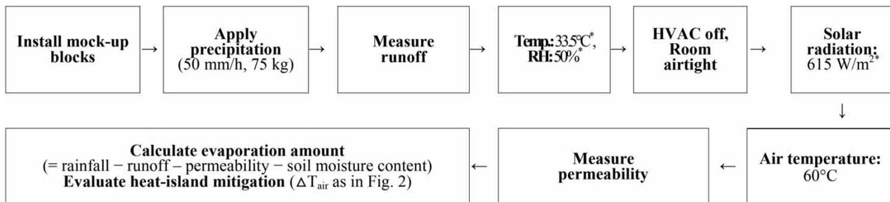
\*Temperature, humidity (RH), and solar data applied based on Seoul standard weather data during heatwave warnings ( $>33^\circ\text{C}$ ) (see Table 4).
