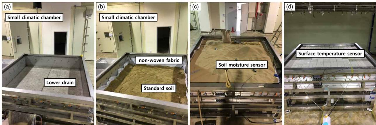
**Figure 3** | Mock-up installation: (a) small climate chamber; (b) addition of non-woven fabric lining and standard soil; (c) placement of soil moisture sensors; (d) placement of test blocks and surface temperature sensors.**Table 5** | Details of the sensors used
