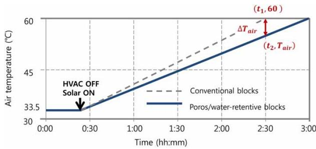
**Figure 2** | Conceptual graph of the heat-island mitigation performance evaluation of two types of blocks.
