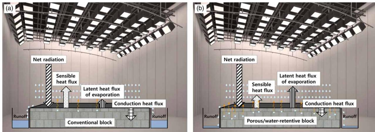
Figure 1 | Heat circulation mechanism of the (a) conventional and (b) porous/water-retentive blocks.
