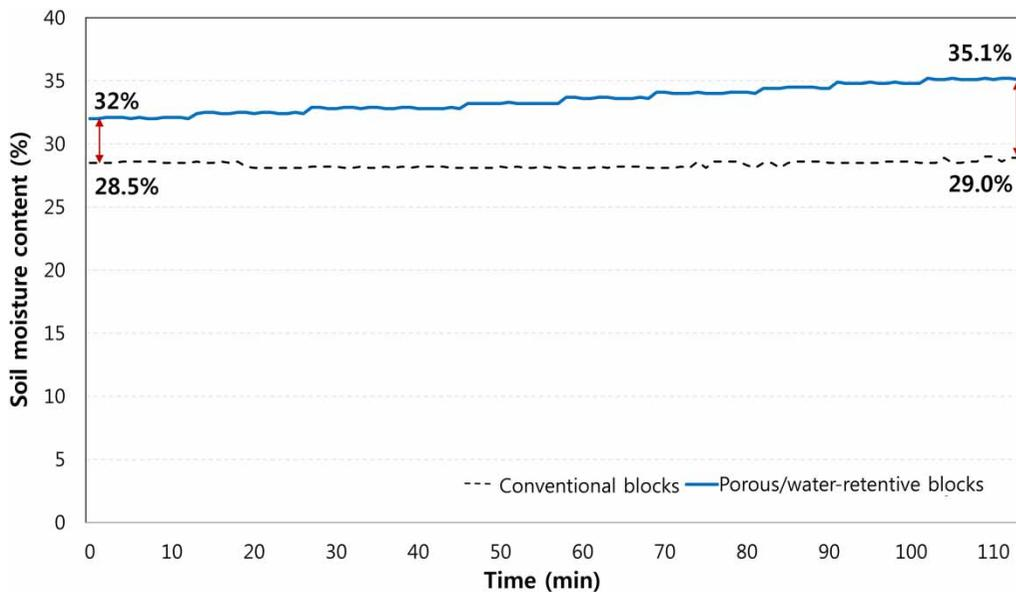
Figure 8 | Soil moisture content below the blocks.
