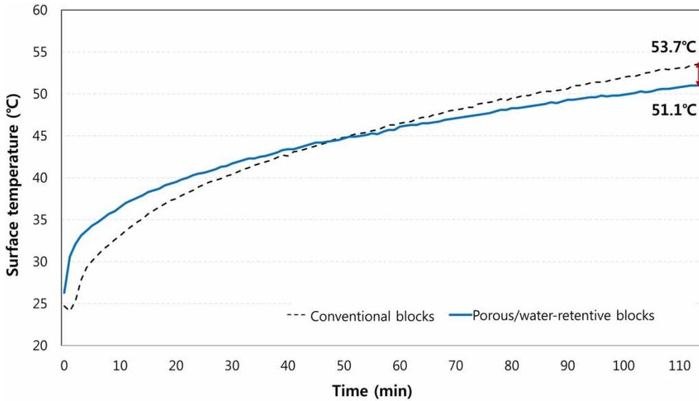
**Figure 6** | Surface temperatures of conventional and porous/water-retentive blocks.
