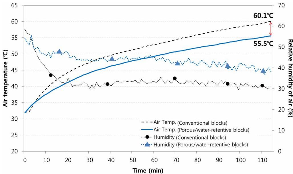
**Figure 5** | Ambient air temperature and relative humidity 50 cm above the tested blocks.
