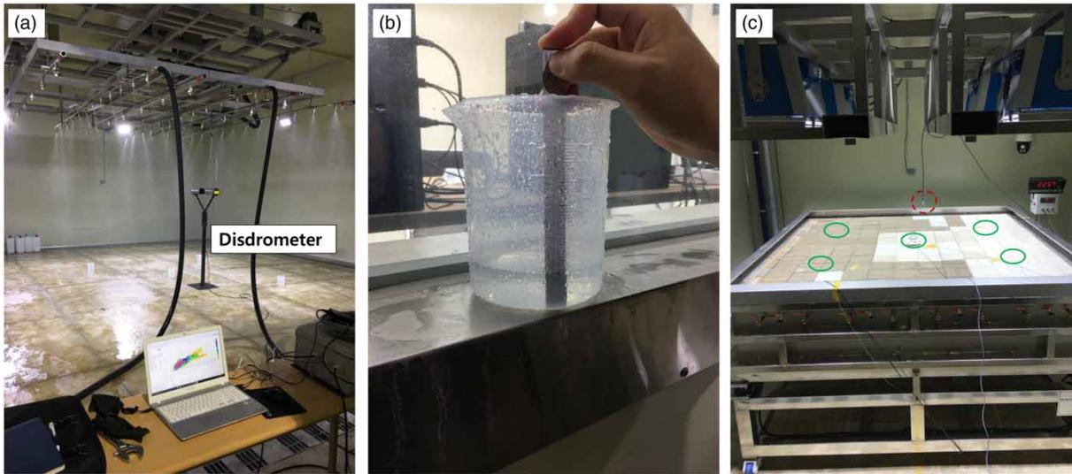
**Figure 4** | Adjustment and measurement processes of (a, b) rainfall using spray nozzles, a laser disdrometer, and rain collection vessels, and (c) solar radiation using lamps, a pyranometer at five points (circles on the blocks) and air temperature (a circle with dotted line above the blocks).
