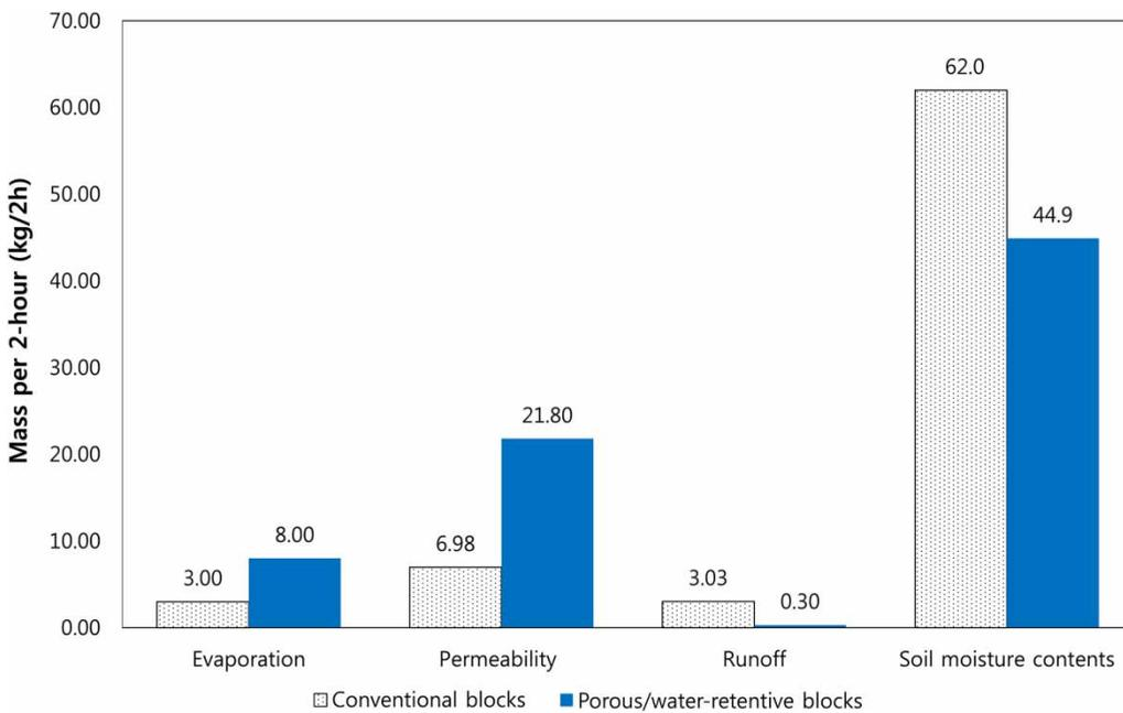
**Figure 7** | Evaporation, permeability, runoff, and soil moisture content of conventional and porous/water-retentive blocks.
