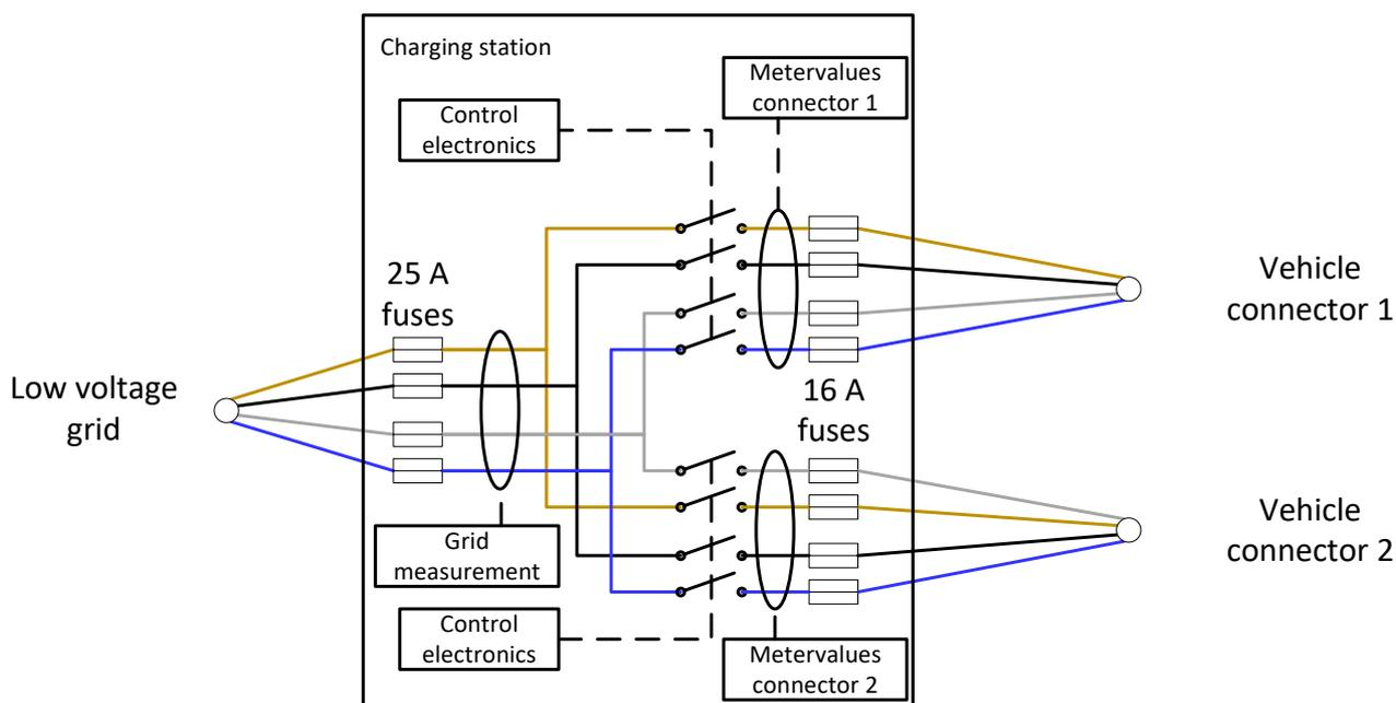
**Figure 3: Protections and phases rotation for the reference charging stations. The wire's order is shifted between the connector 1 and 2.**
