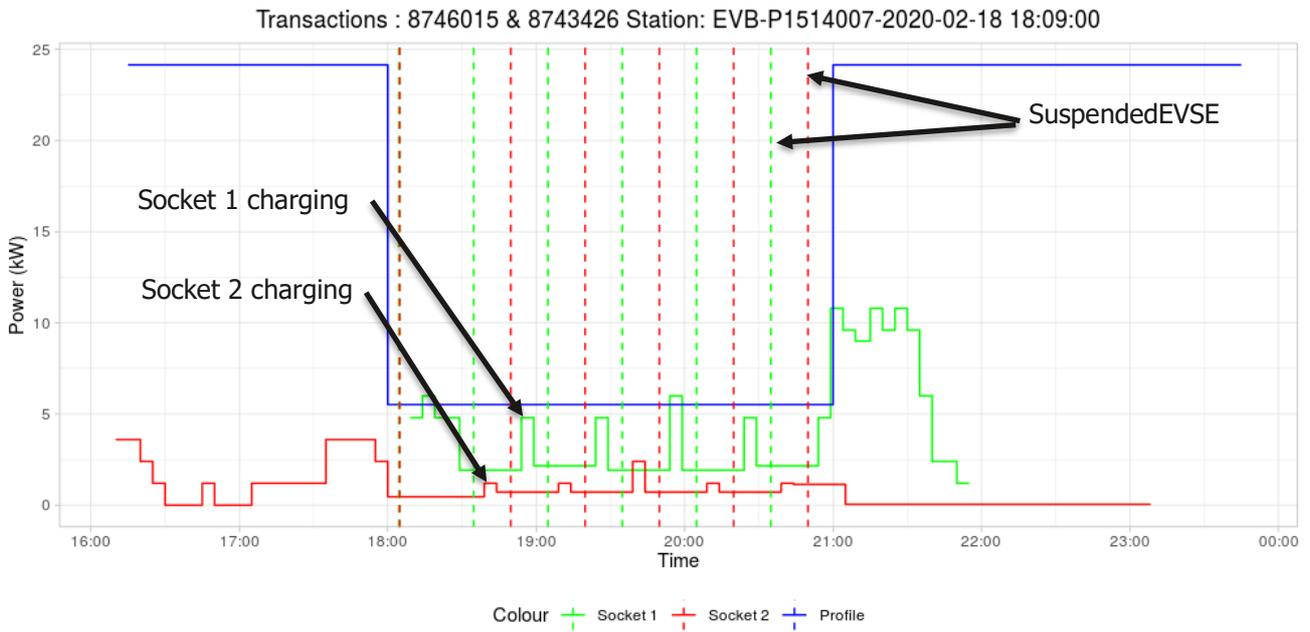
**Figure 6: Example of alternating charge. Two vehicles are simultaneously connected to a charging pole. During the restricted period, the current values alternates between the two sockets. The value doesn't go down to 0 because the measured period is not synchronised with the actual current. The energy and thus the power are an average on the time interval.**
