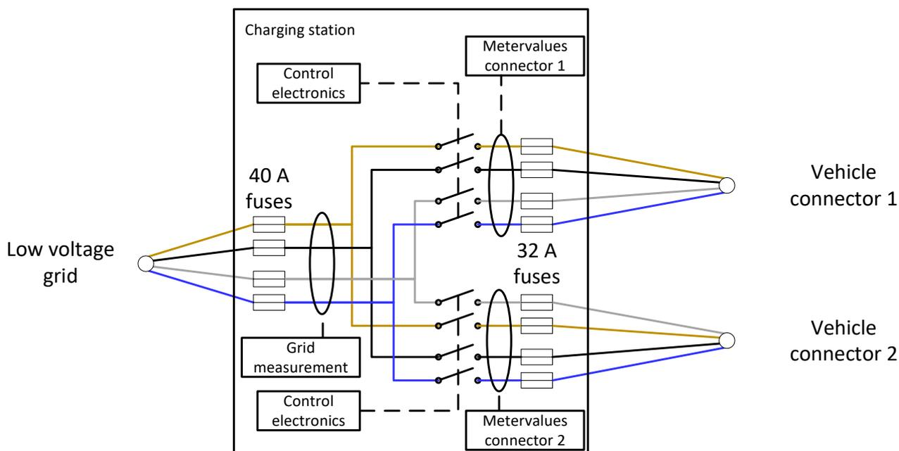
**Figure 4: Protections and phases rotation for the Flexpower 1 charging stations**
