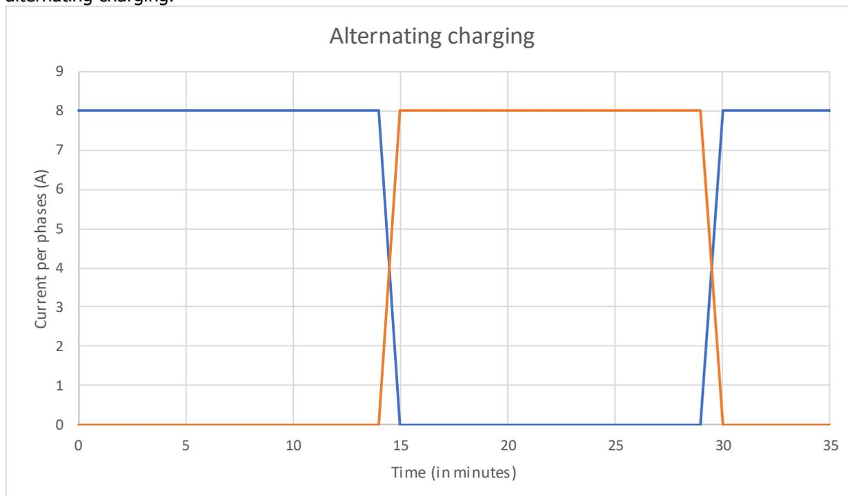
**Figure 5: Illustration of the current swing during alternating charging.**
