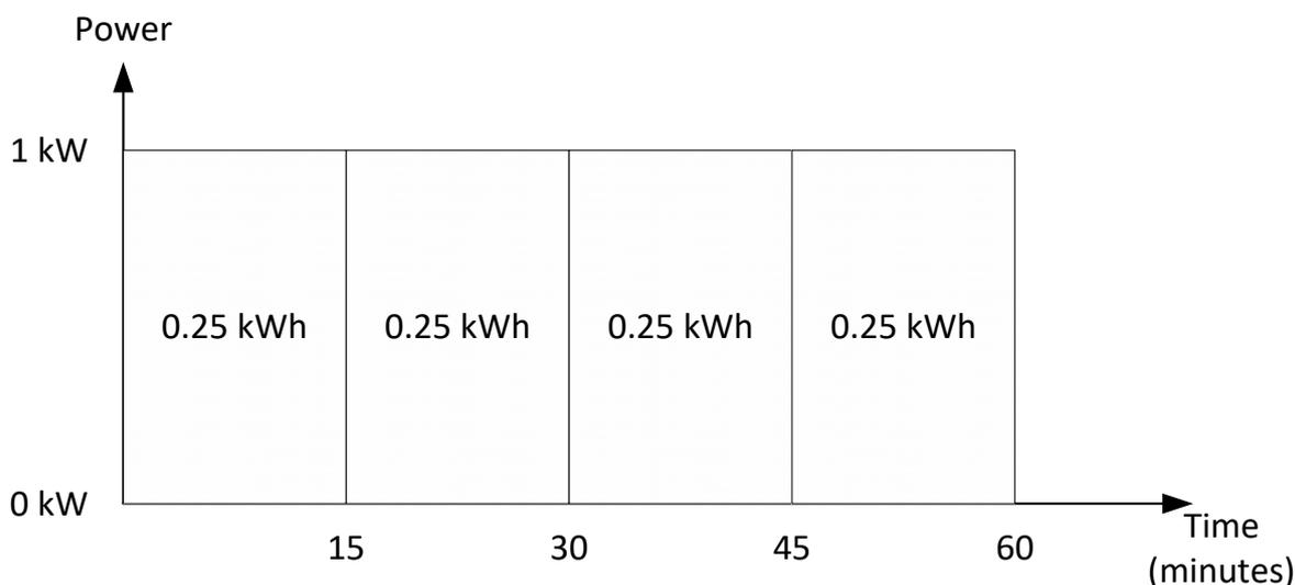
**Figure 2: Even of the power is constant, the energy will vary according to the duration it is applied.**
