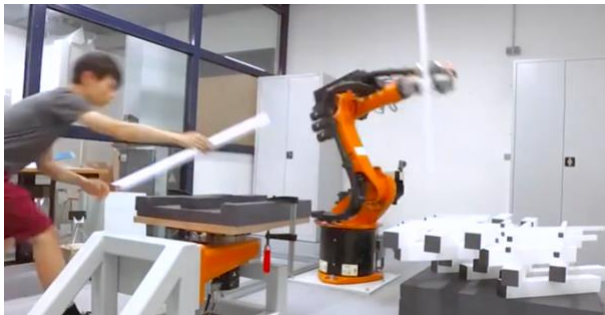
Figure 5. Huma-robot stacking of linear elements tested in lab conditions
