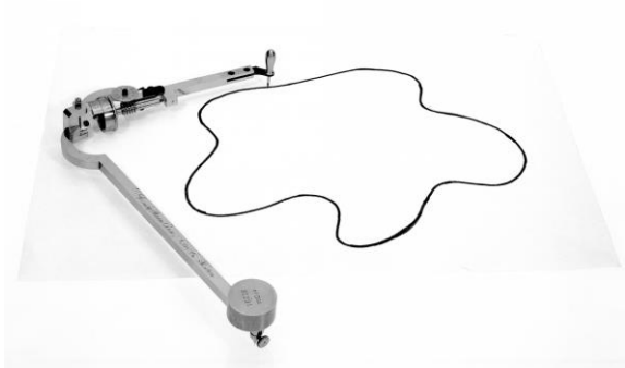
Above: Amsler Type 2 Polar Planimeter, Sold by Crosby Steam Gage & Valve, 1880s. Courtesy of the Smithsonian Institution's National Museum of American History.
