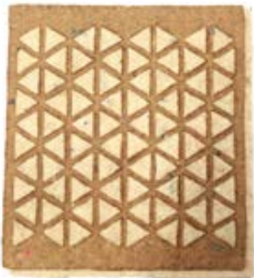
Jute and PLA Laser cutting combining hard and soft
