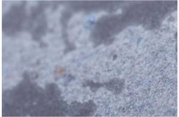
Cotton dust from filter and Cradonyl (PLA/TPS) hot pressed
