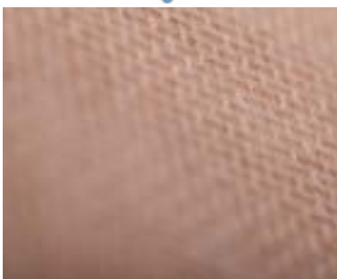
Woven jute with Solanyl (TPS-based bioplastic) hot pressed
