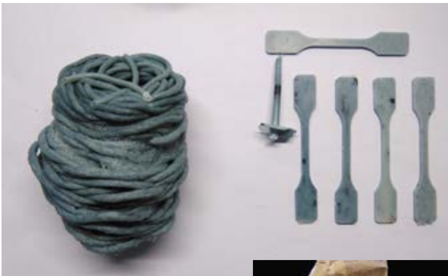
Denim and PLA/TPS Injection moulded
