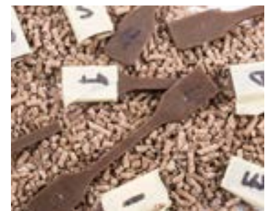
Pulverised jute with PLA tension bar plus granulate
