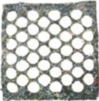
Denim and PLA Laser cutting before pressing
