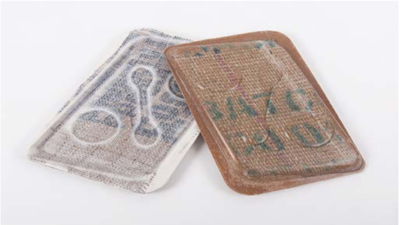
Serving trays made from a.o. jute mats and Solanyl (PLA/TPS) Hot pressing
