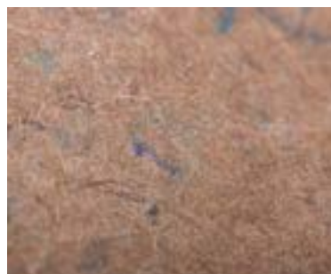
Fiberised and needle punched jute and PLA hot pressed
