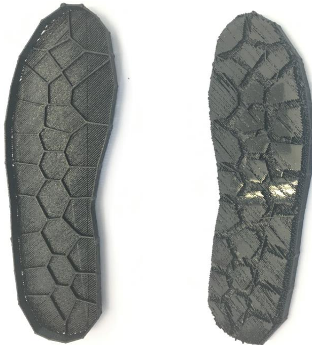
Fig. 8: Top view and bottom view of 3D printed sole in Filaflex as generated by Sole Maker.
